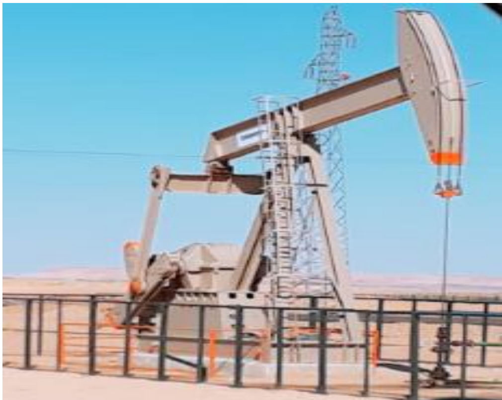
Figure II.1. Le pompage aux tiges.
