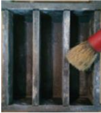
Figure II.29 : Lubrification des moules (4 x 4 x 16) cm.
