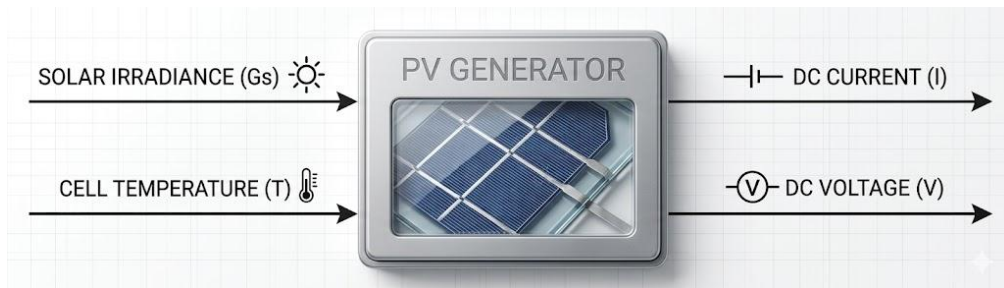
Figure I.6. Block Diagram of a PV Generator
