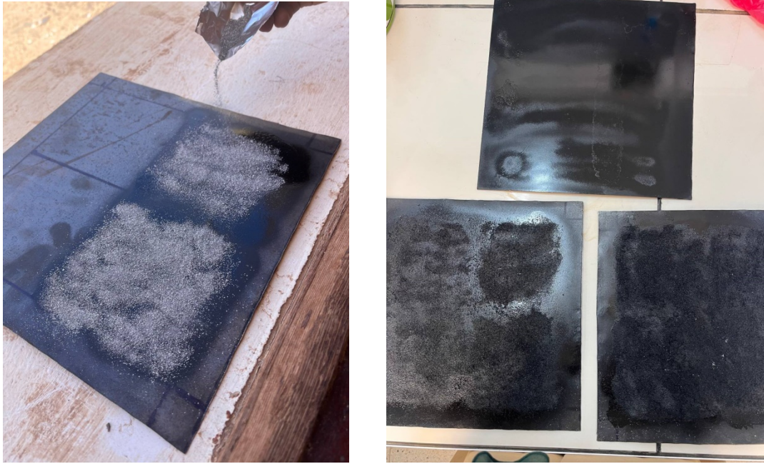
Figure II.11: Method of placing filings aluminum
