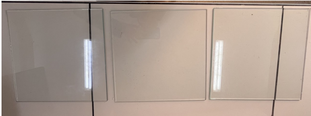
Figure II.4 : Explicit view of the 5 mm transparent glass covers prepared for installation
