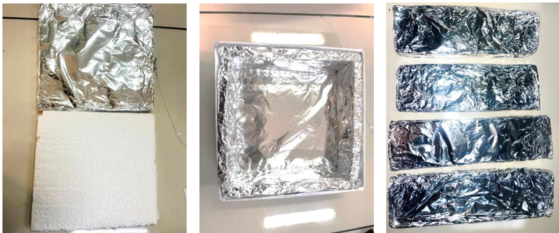
Figure II.3: Internal lining displaying the polystyrene insulation layer layered with protective aluminum foil
