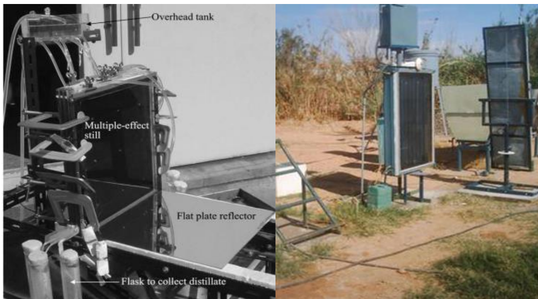
Figure (2.5): Multiple-effect basin type diffusion-coupled solar still (Tanaka et al., 2009).
