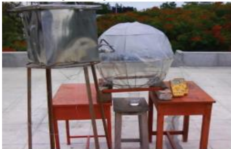
Figure (2.8): Pictorial view of spherical solar still (Arunkumar et al., 2012).
