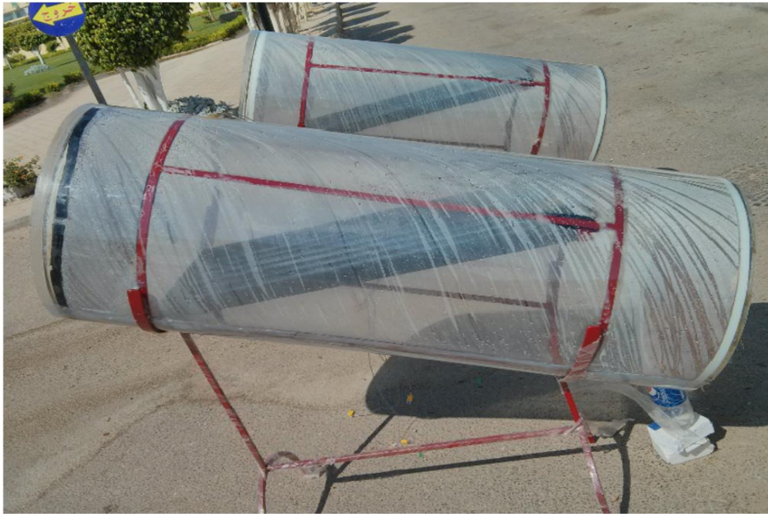
Figure (2.10): Photo of tubular solar still model (Elshamy et al., 2018).
