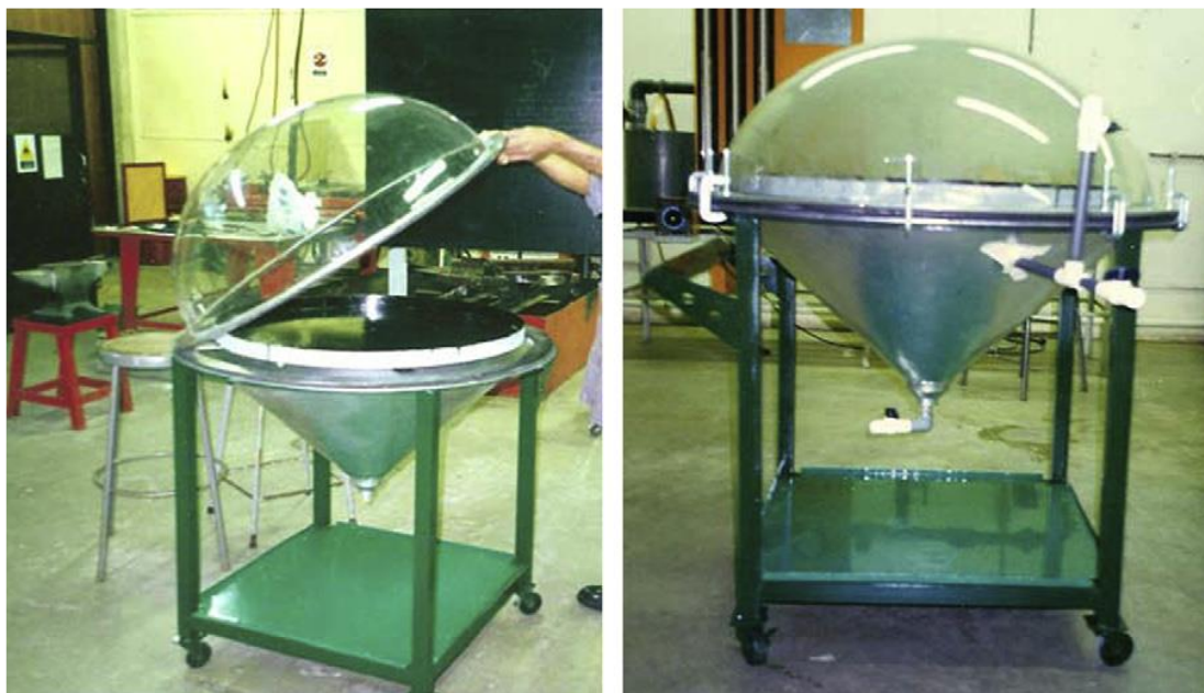
Figure (2.14): Photographs of the fabricated hemispherical solar still (Ismail, 2009).
