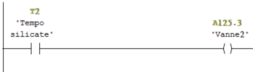
Figure 4-9 La temporisation T2 silicate
