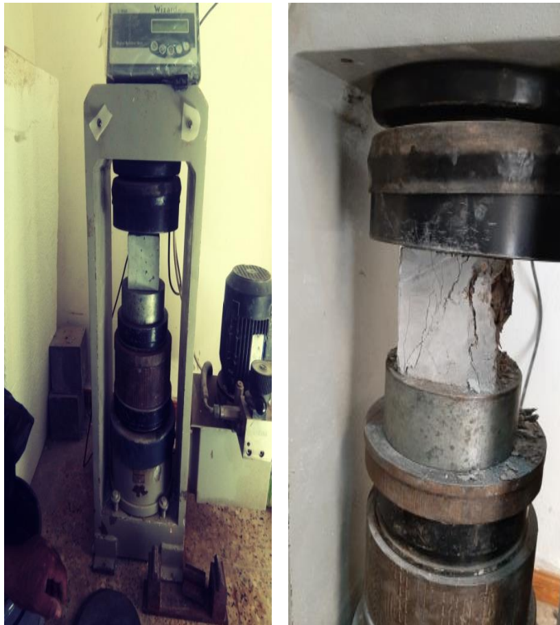
Figure III.3. essai de compression
