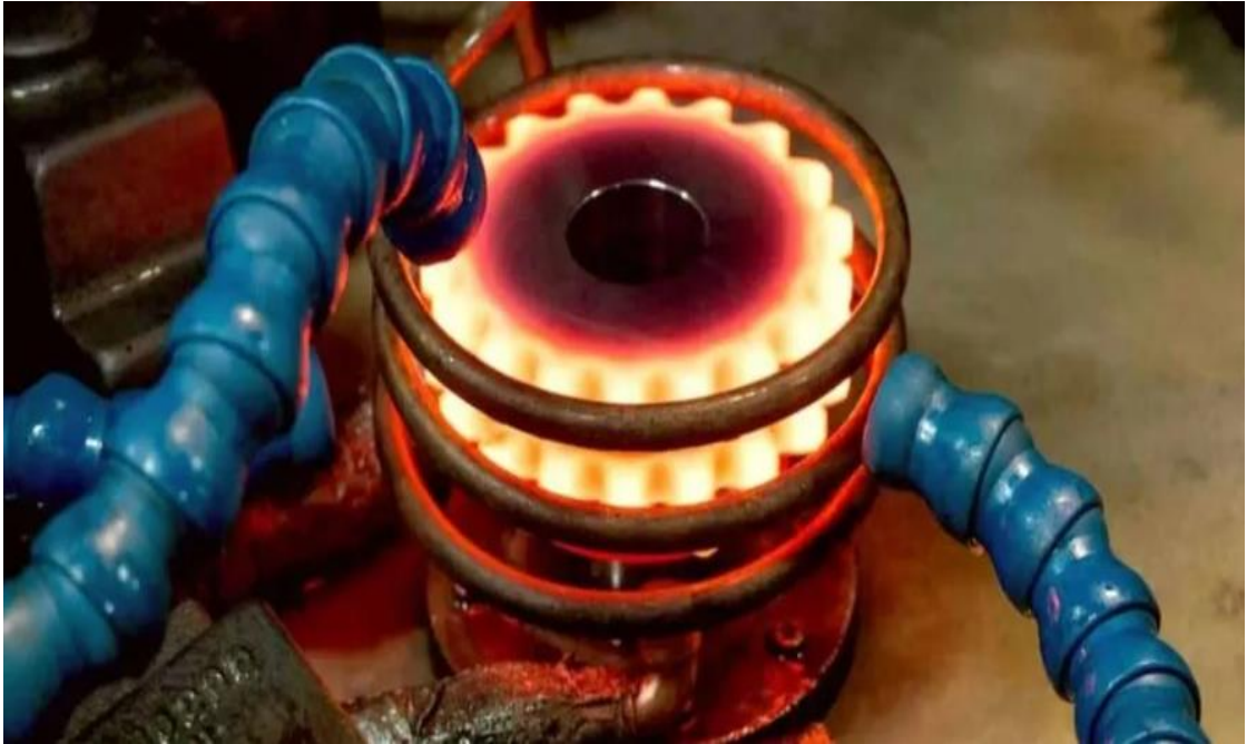
Figure II.21: Surface Heat Treatment.[20]
