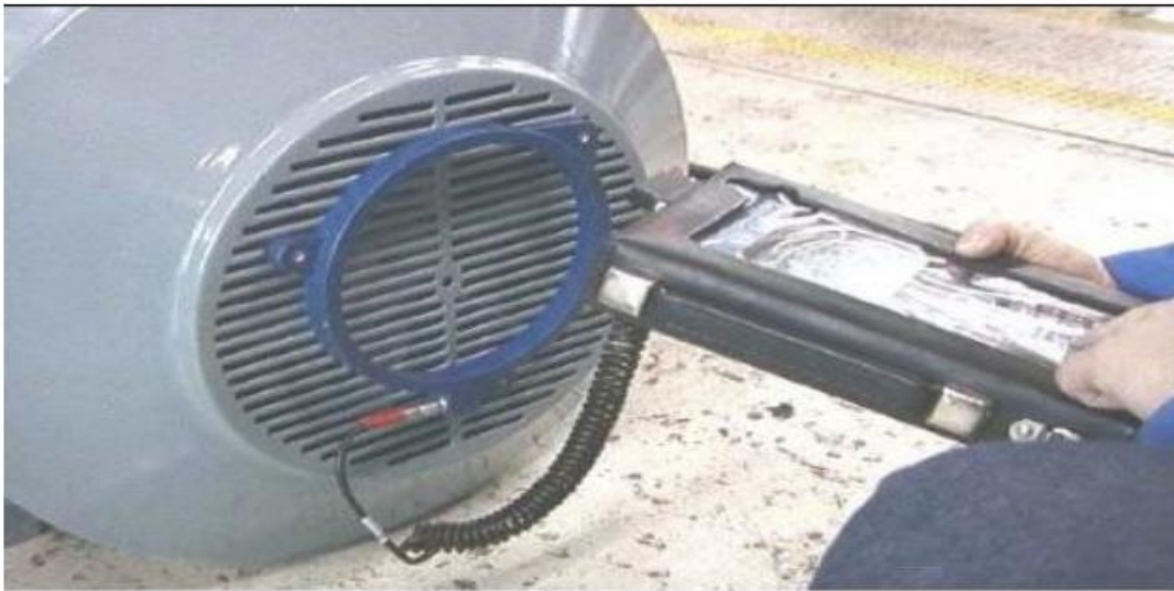
Figure (I.13): Measurement of axial flux [26].
