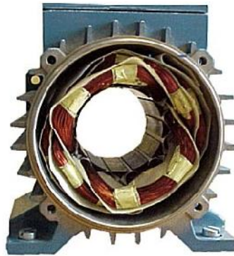
Figure 1.2: Stator d'une machine asynchrone.
