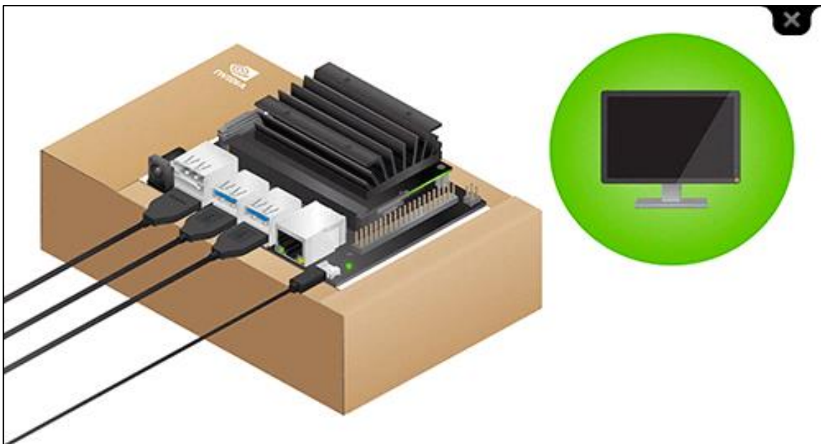
Figure 3. 4: Jetson Nano Setup with Display Attached.
