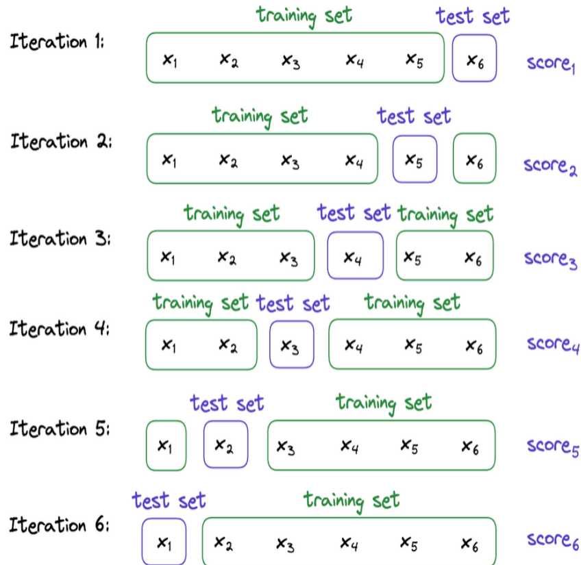
Figure 2.14: Example: For a dataset with 6 samples, we perform 6 iterations. In each iteration, one different sample is used for testing: S_1 = \{x_1\} , S_2 = \{x_2\} , \dots , S_6 = \{x_6\} .
