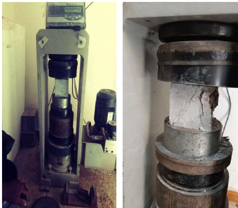
Figure III.4. Essai de compression.
