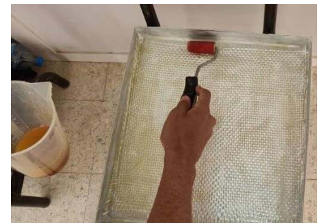
Figure III.10. Impregnating the fabric layers with resin
