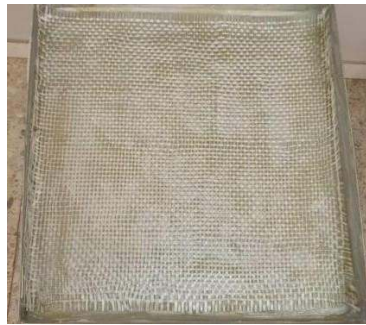
Figure III.9. Placing the fabric layers
