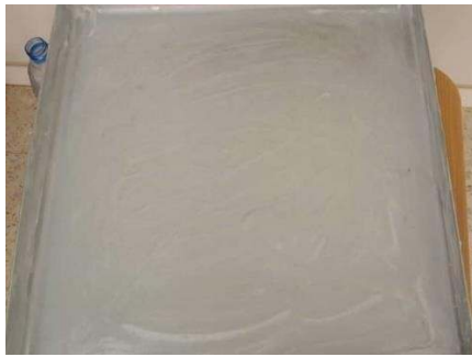
Figure III.8. a release agent on the mold plate
