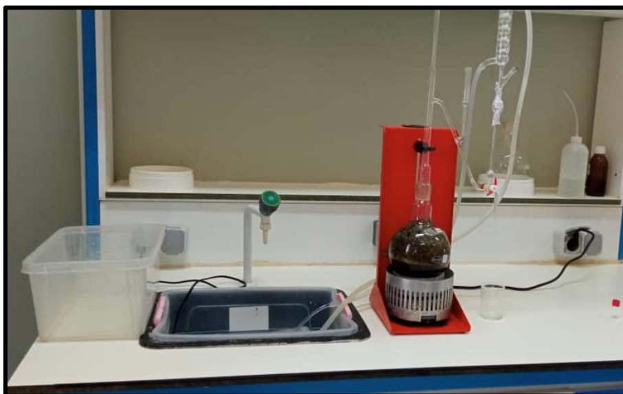
Figure 25. Photo represent the extraction device type Clevenger for Essential oil of aquatic Mentha (Original, 2024).
