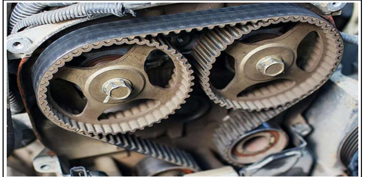
Figure II.2: The distribution belts[31].
