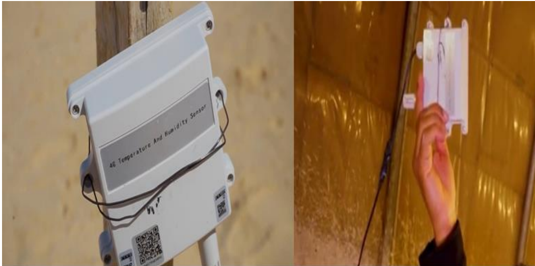
Figure 12 : The device in the picture is used to measure temperature and humidity and transmit data via 4G internet.
