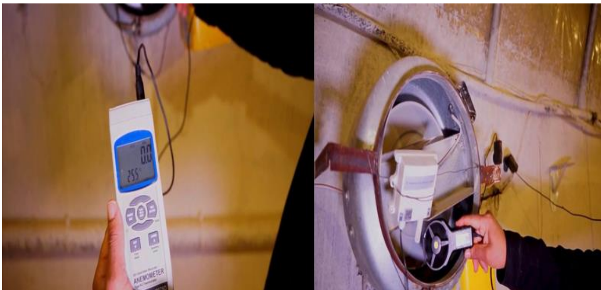
Figure 11 : The device in the picture is used to measure temperature and air velocity.
