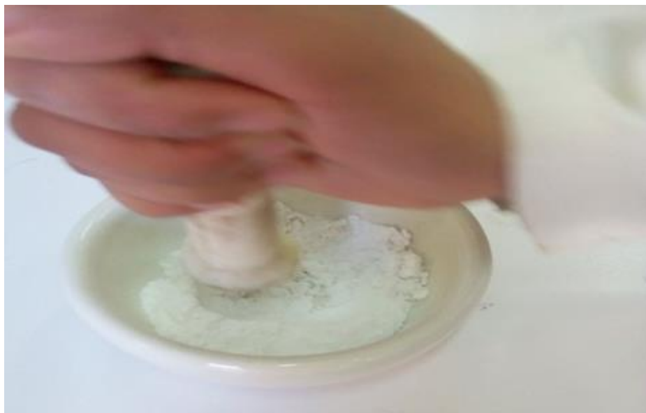
Figure III. 4: Processus de broyage
