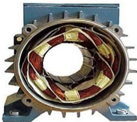
Figure (I-2) le stator de la MAS
