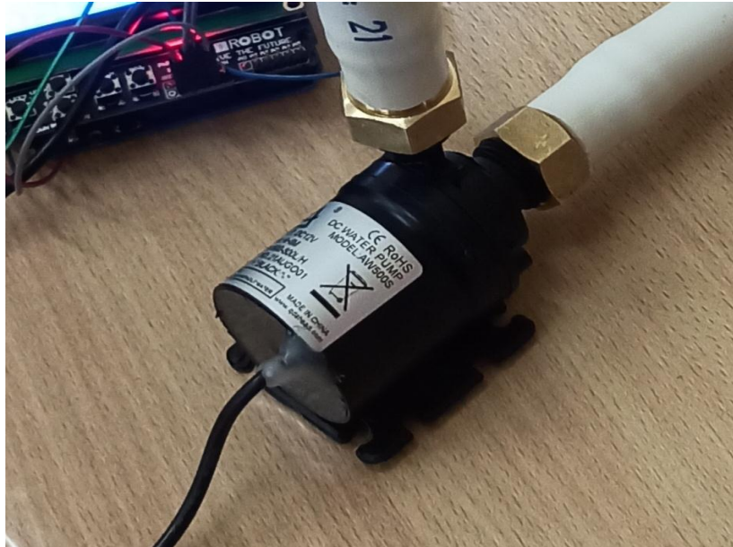
Figure III. 4: pompe a eau
