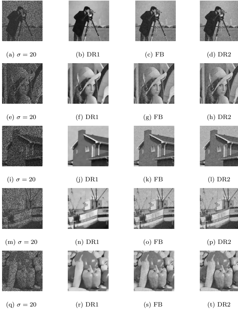
Fig. 2: Restored images with different proximal algorithms ( \sigma = 20 ) for 'cameraman', 'lena', 'house', 'boat' and 'peppers'.
