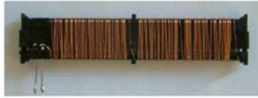
Figure 2. 6: Antenne ferrite ( n = 160 tours, \mu r = 60 , L = 820 \mu H )
