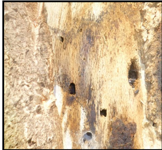
Figure 27: Trous d'insecte xylophage (Original)
