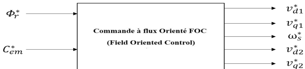
Figure III.8: Simplified block diagram of flux oriented control (FOC)
