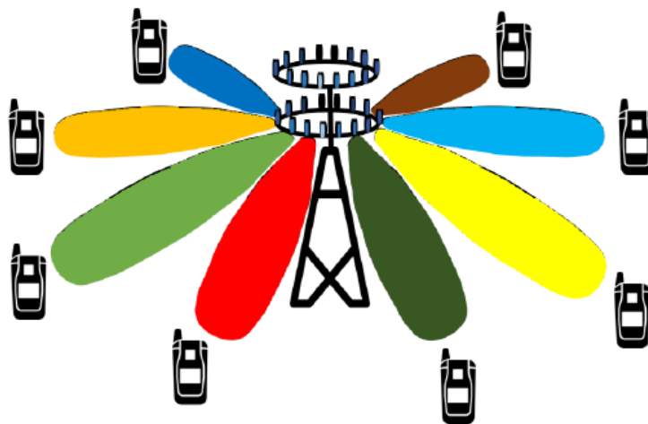
Figure II.5. Massive Multiple Output–Multiple Output (MIMO) beamforming. [11]
