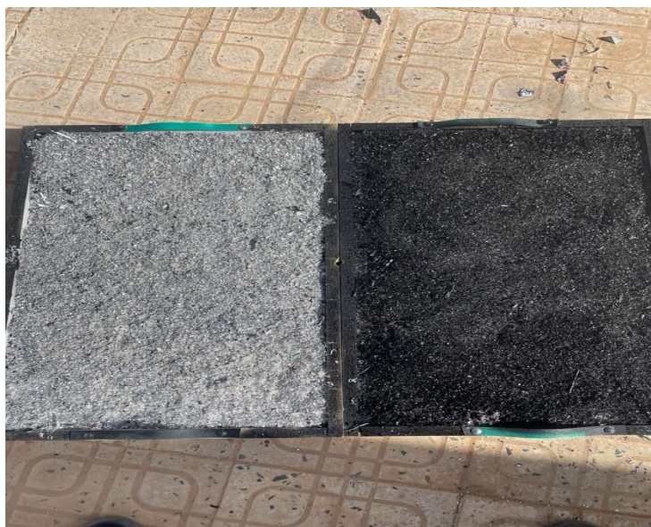
Photo III (13): salt and Aluminum filing mixture before and after painting
