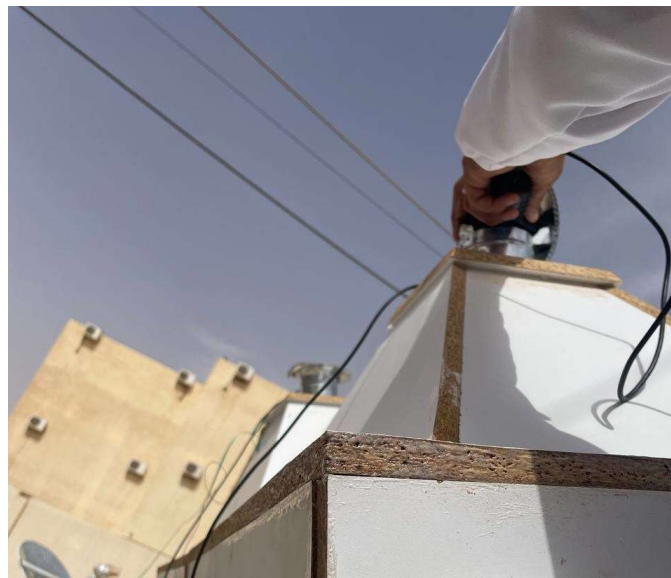
Photo III (16): inlet airflow measurement
