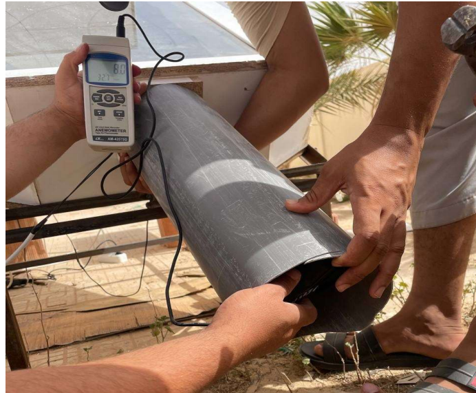
Photo III (16): inlet airflow measurement
