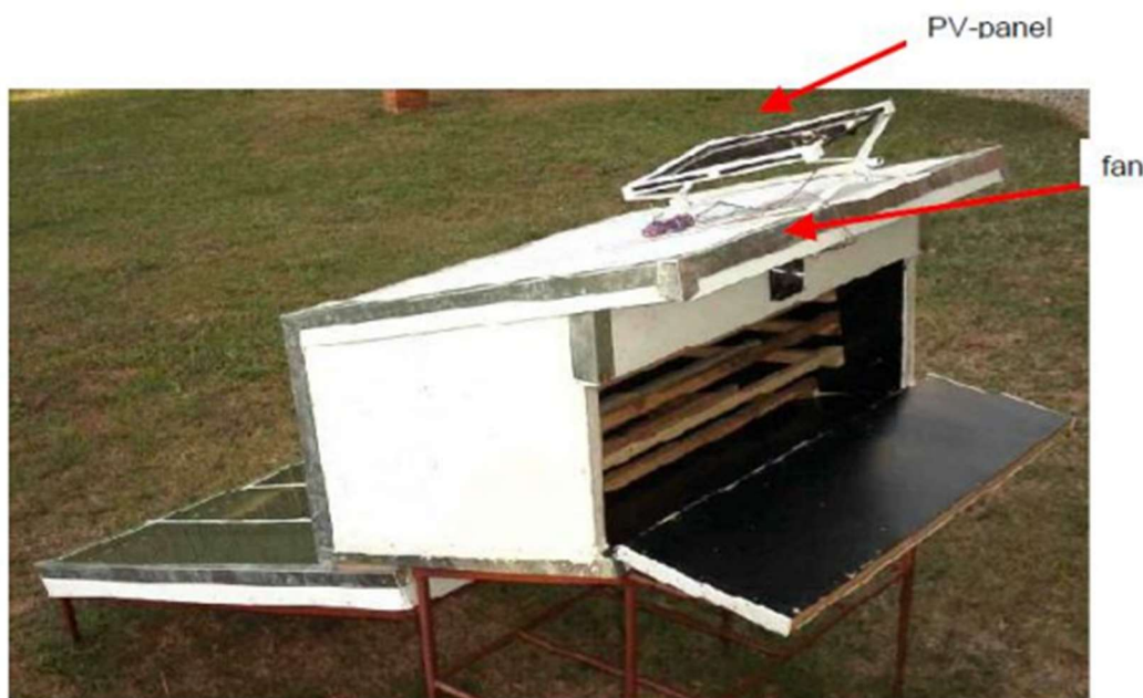
Figure II.5: Fan powered by photovoltaic panel.
