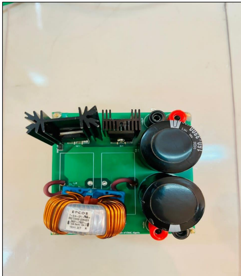
Figure VI.16: Real photo of Buck-Boost converter board.
