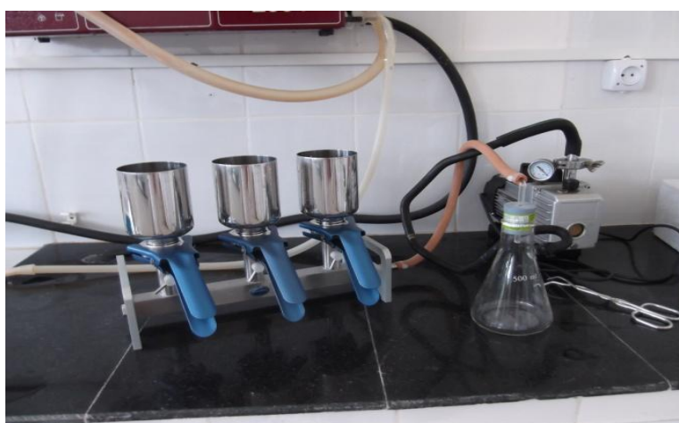
Photo V.6: Ensemble de filtration (ONA, 2015).
