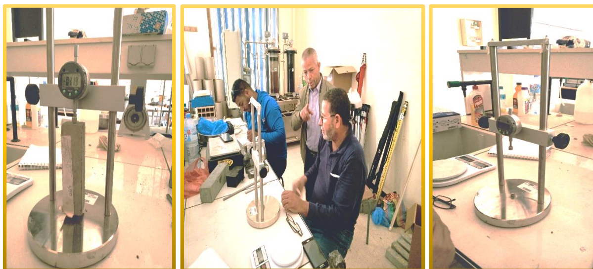
Figure III.22: Essai de Retrait.
