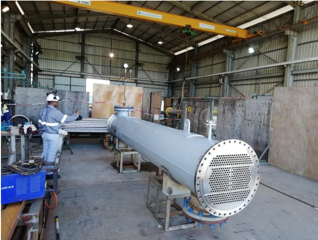
Figure 1.1. Heat exchange in the workshop
