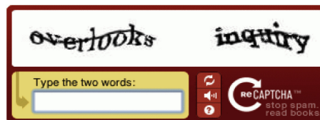
Figure 3.5: ReCAPTCHA. A text-based CAPTCHA and book digitization project that requires the user to interpret two visually distorted meaningful words and type them into a response box.
