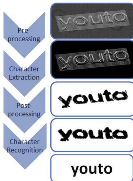
Figure 3.7: Overview of the stages.
