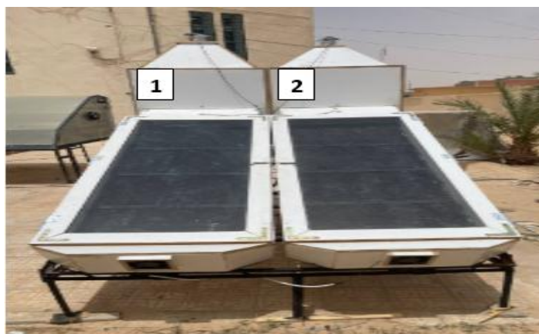
Figure (III- 29): séchoir solaire indirect
