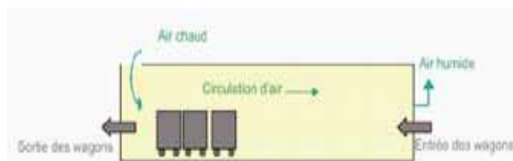
Figure (II- 11): le séchoir tunnel [43]
