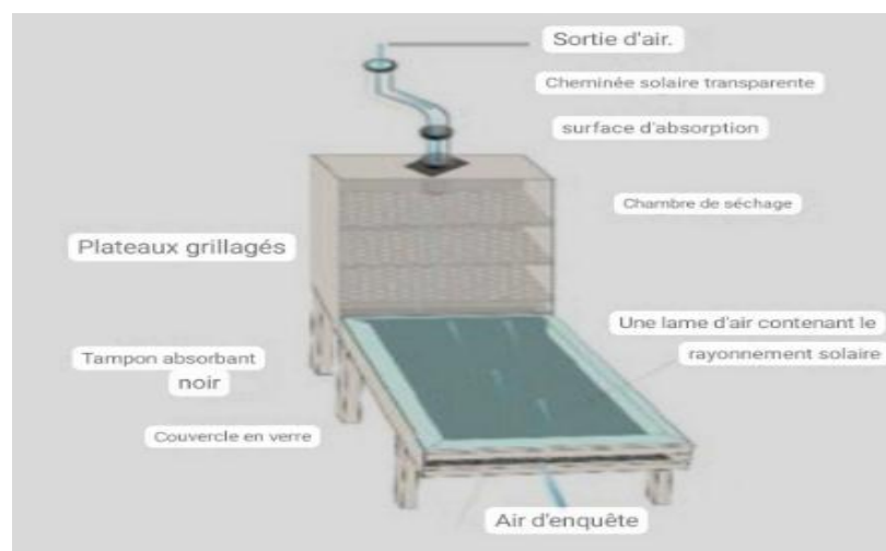
Figure (II- 14): Séchoir solaire indirect passif [45]
