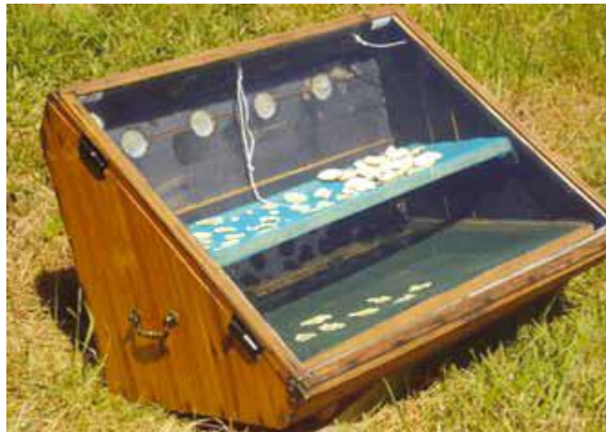
Figure (II- 12) : Séchoir solaire direct portable. [43]
