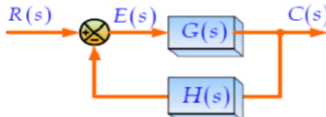
Figure 5.2 closed-loop control system
