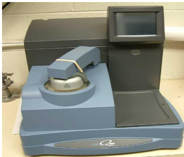
Figure II.6: Machine DSC de marque DSC Q800.
