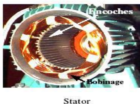
Figure(I.2): Stator de la machine asynchrone
