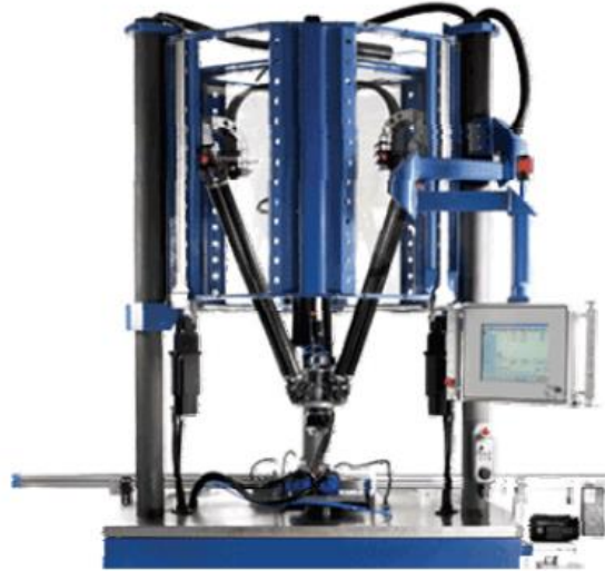
Figure I.18. Manipulator using the Delta architecture with linear actuators
