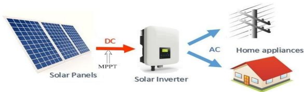
Figure I.22: the renewable energy inverter DC to AC
