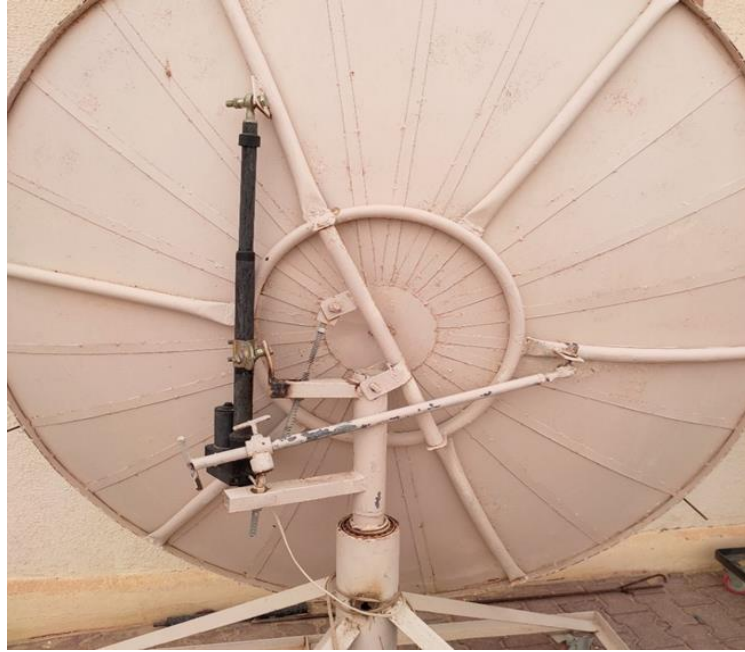
Figure II. 5: Photo of the tracking system containing a cylinder and a rotary axis.
