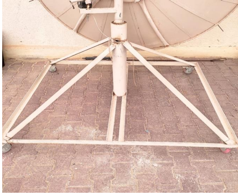
Figure II. 4: Photo of oven support structure.
