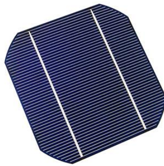
Figure II-1: cellules en silicium monocristallin [13]
