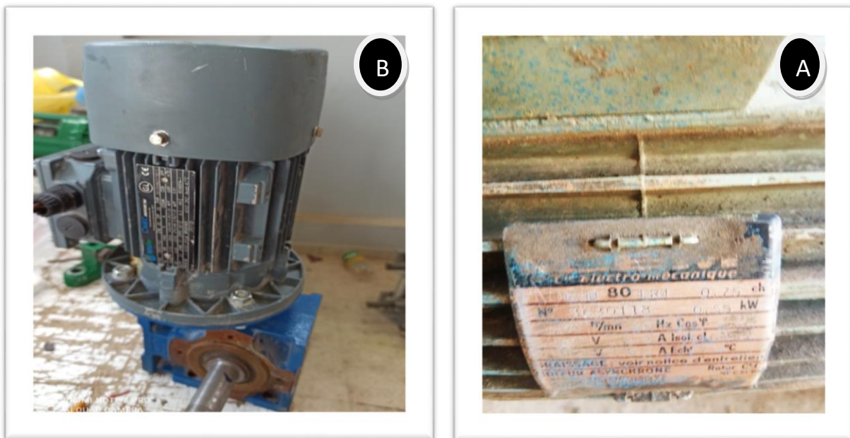
Figure III.16. Three Phase Asynchronous Motors
