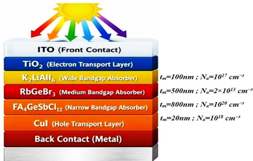
Figure 3.10: Optimal Device Configuration of the Trilayer Absorber PSC.
