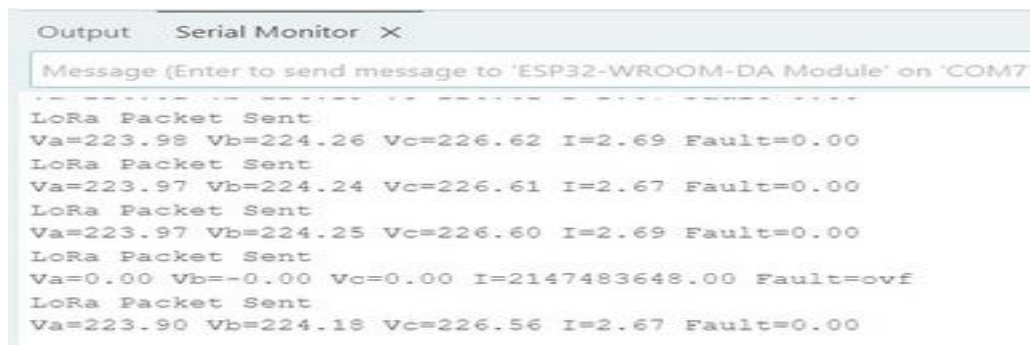
Figure 3.31: The 1 st ESP32(Node) serial monitor readings(Healthy state).
