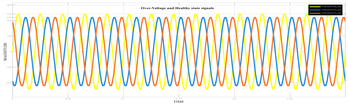
Figure 2.7: Three-Phase Voltage Signals during Over-Voltage Detection
