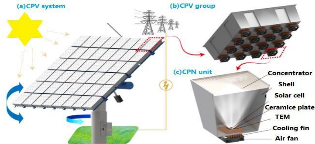
Fig.I.13. Conceptual schematic of the self-cooling concentrated photovoltaic system[26]
