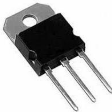
Fig.III.38. The SWITCHMODE Power Rectifi
