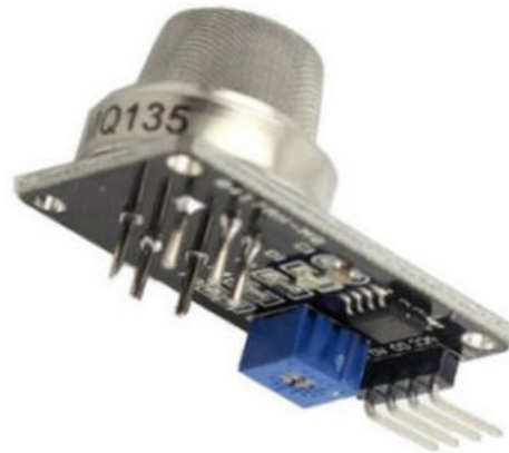
Figure 4.4: Air quality sensor
