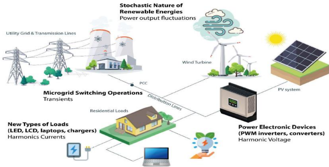
Fig.1.1. Sources of power quality disturbances in microgrid [5] .
