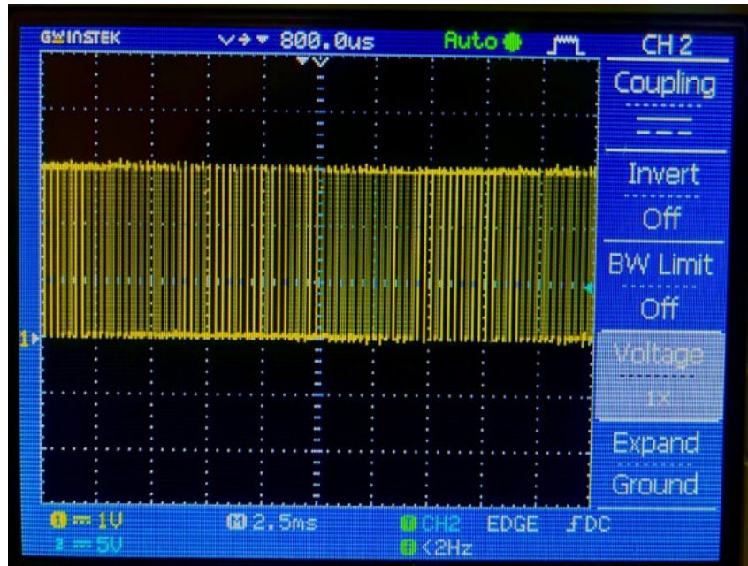
Figure 3.12: the Sinusoidal Pulse Width Modulation signals
