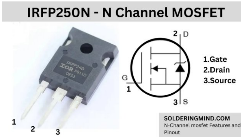
Figure 3.4: The IRFP250N Power MOSFET [12].
