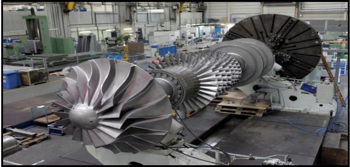
Fig.III.15. Industrial View of a Centrifugal Compressor Rotor Supported by Magnetic Bearings [3].
