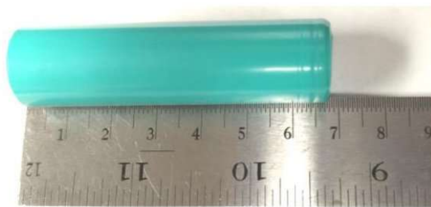
Figure (2-6): INR 18650-20R Battery
