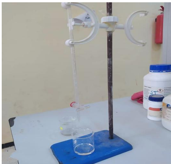
Figure 21: Titration of acrylic acid with sodium hydroxide to modify pH.
