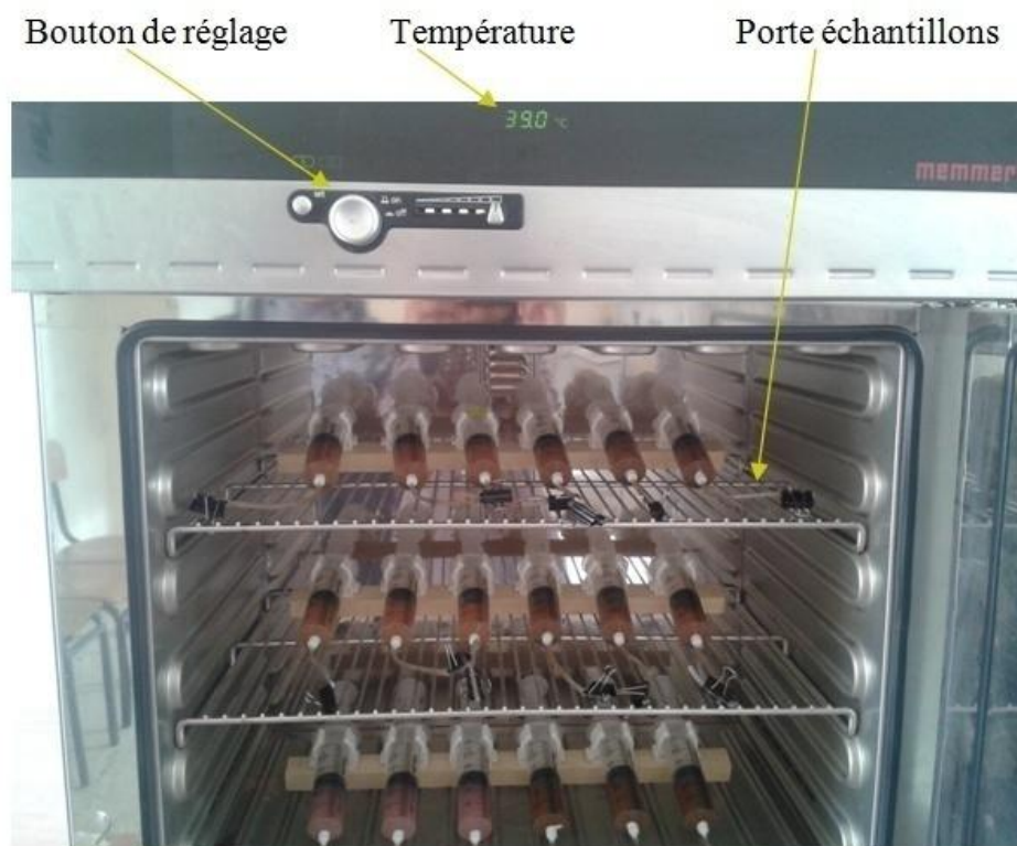
Figure 13: Etuve (type MEMMERT) (photo originale).
